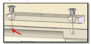
Step 3: Inspect the inside of the receiver to confirm the end of the torx screw does not interfere with the bolt.
